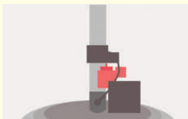
1 A cut-off safety switch disconnects the motor in the event of a fan mounting failure.
